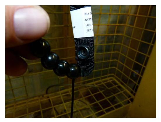
4. The additional stitch prevented the cord from pulling out from underneath the press stud and added an additional 20kg's strength to the units.
