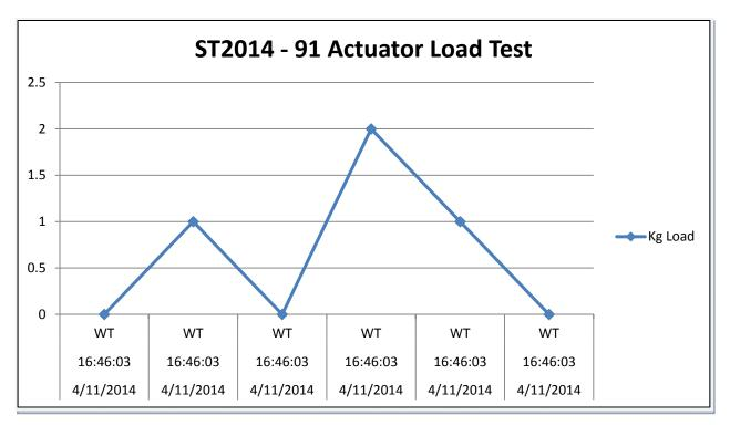
Graph needed to be plotted in XL as all readings took place in .03 of a second. Unit snapped out of plastic housing at 2kg as it was not the complete unit fixed in the vest.
